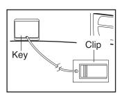
key into the console. **IMPORTANT: In an emergency, the key can be pulled from the console,** causing the walking belt to slow to a stop. Test the clip by carefully taking a few steps backward; if the key is not pulled from the console, adjust the position of the clip.
